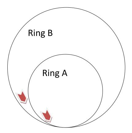
Ring B is for full size narrow bodies. Nominal radius 3-3.5 NMi Ring A is for light weight, jet and turboprop, Nominal radius 2-2.5 NMi
